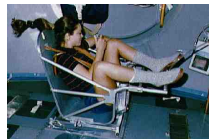
e / Astronaut Tamara Jernigan measures her inertial mass aboard the Space Shuttle.
